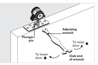
Note: The top of the hanger shaft screws into a selflocking nut. If the hexagonal nut is turned downwards too far, the shaft will become loose from the selflocking nut. If the turning resistance suddenly feels much easier, you have gone too far.
