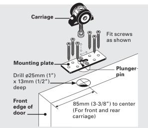
d) Mount bearings at the bottom of each door using the screws supplied.
